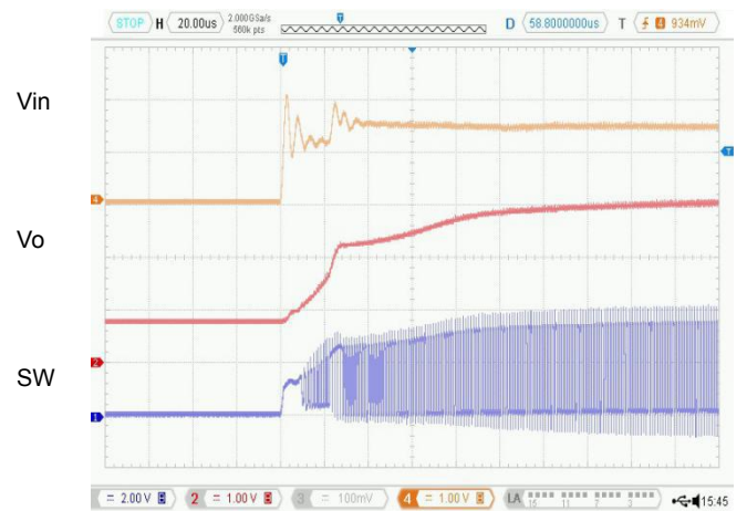
6. Start-up Waveform(VIN=2.4V, Rs=0.12Ω)
