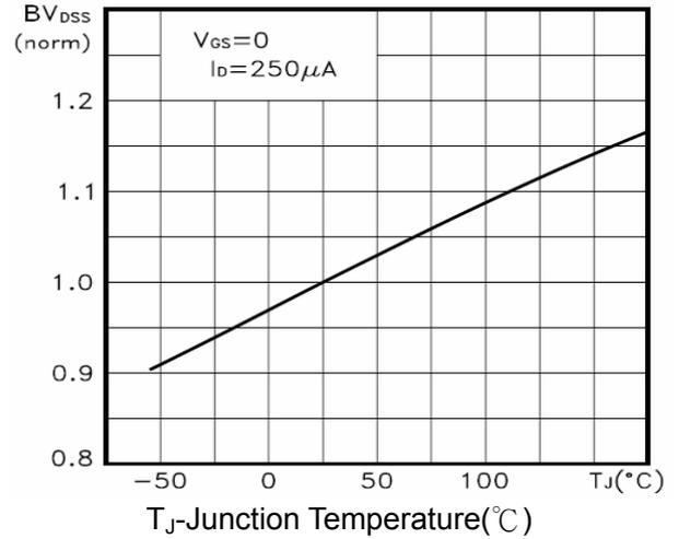
Figure 9 BV<sub>DSS</sub> vs Junction Temperature
