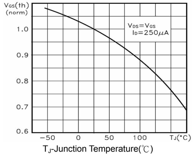
Figure 10 V<sub>GS(th)</sub> vs Junction Temperature
