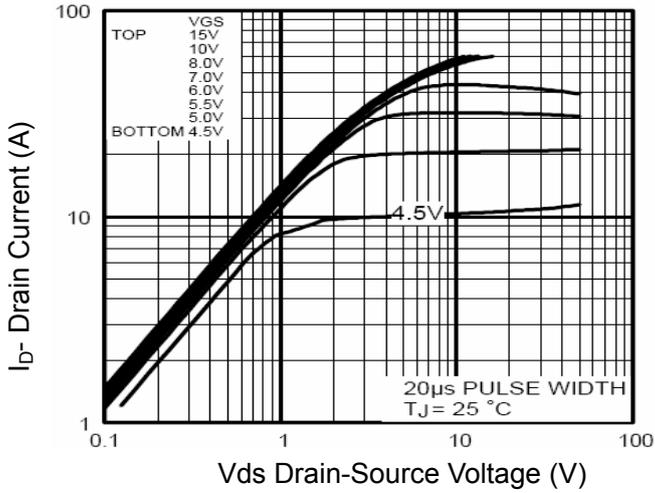
Figure 1 Output Characteristics
