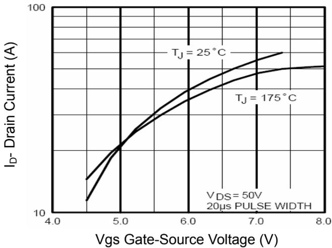
Figure 2 Transfer Characteristics
