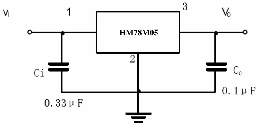
\*Bypass capacitors are recommended for optimum stability and transient response and should be located as close as Possible to the regulators.
