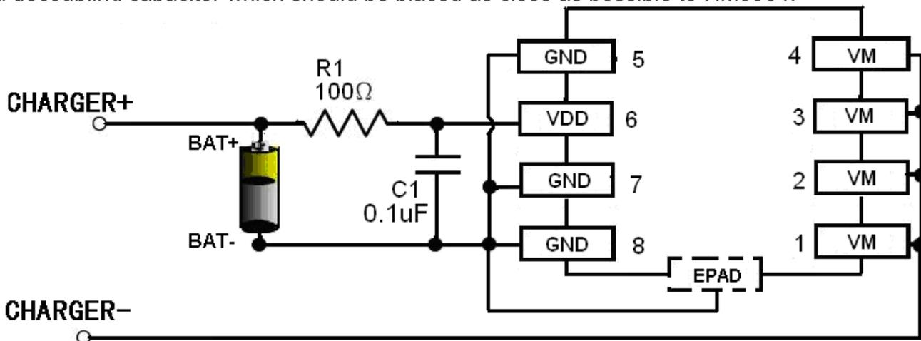
Fig 6 HM9904 in a Typical Battery Protection Circuit
