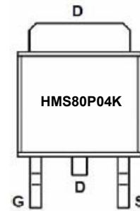
Marking and pin assignment
