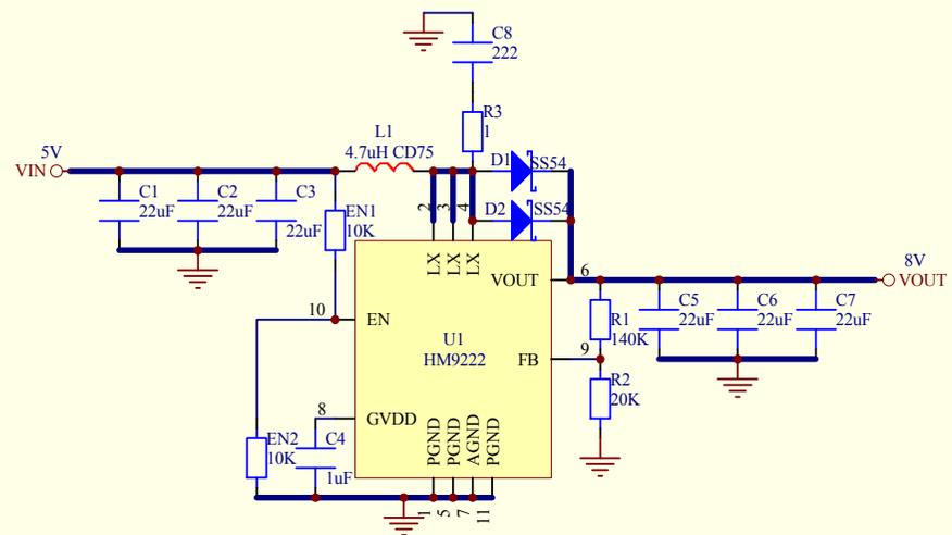
\*输出电压设置:  $V_{OUT} = 1V * (R1/R2 + 1)$
