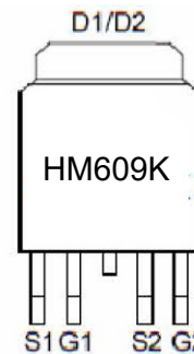
Marking and pin assignment
