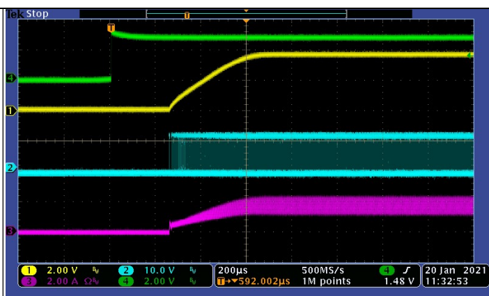
Fig 8 Enable Start up ( V_{in}=12V , V_{out}=3.3V , I_{LOAD}=2A )
