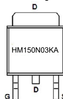
Marking and pin assignment
