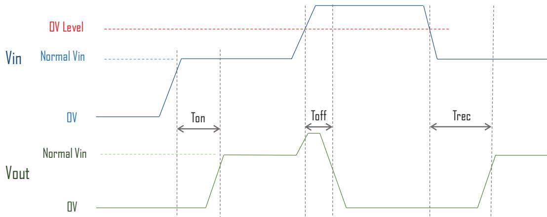
$T_{on}$ : the time from 90%  $V_{IN}$  at  $V_{IN}$  terminal to 90%  $V_{OUT}$  at  $V_{OUT}$  terminal
